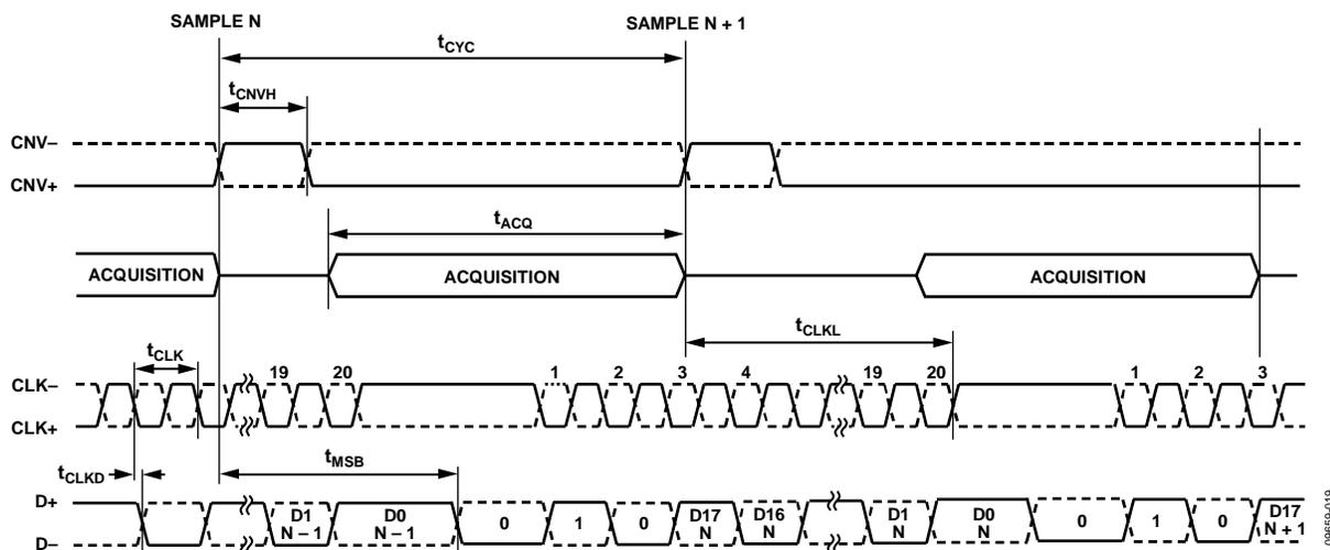
Figure 36. Self Clocked Interface Mode Timing Diagram
