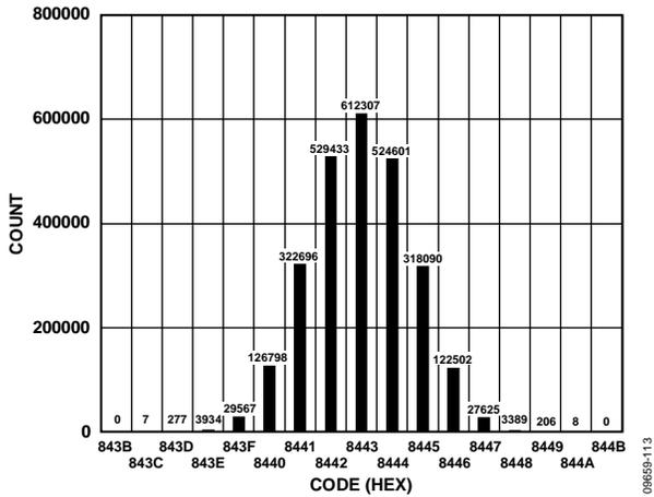
Figure 11. Histogram of DC Input at Code Center, REF = 4.096 V
