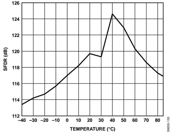
Figure 22. SFDR vs. Temperature, REF = 5 V
