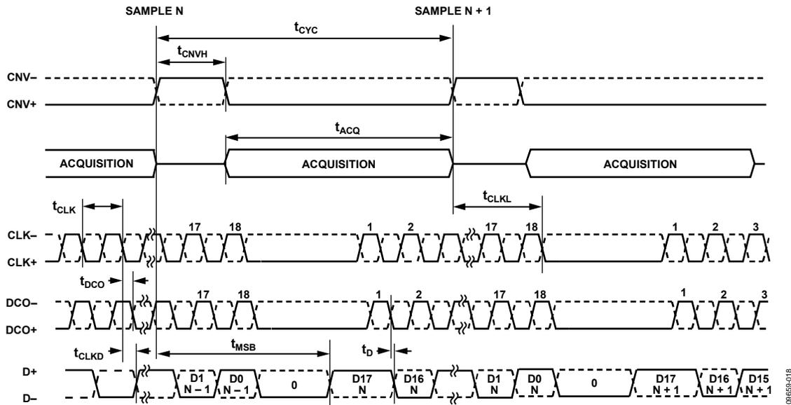
Figure 35. Echoed Clock Interface Mode Timing Diagram
