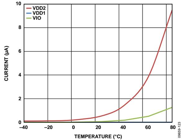
Figure 26. Power-Down Current vs. Temperature, REF = 5 V
