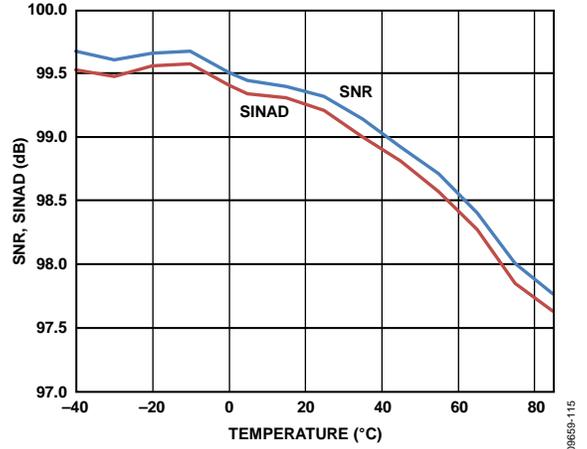
Figure 20. SNR and SINAD vs. Temperature, REF = 5 V
