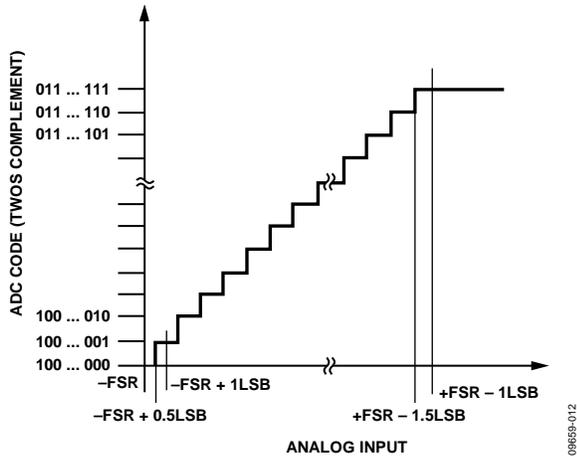
Figure 29. ADC Ideal Transfer Functions (FSR = Full-Scale Range)
