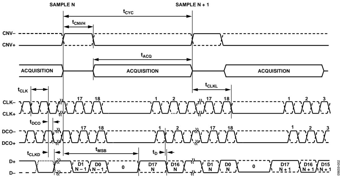
Figure 2. Echoed Clock Interface Mode Timing Diagram
